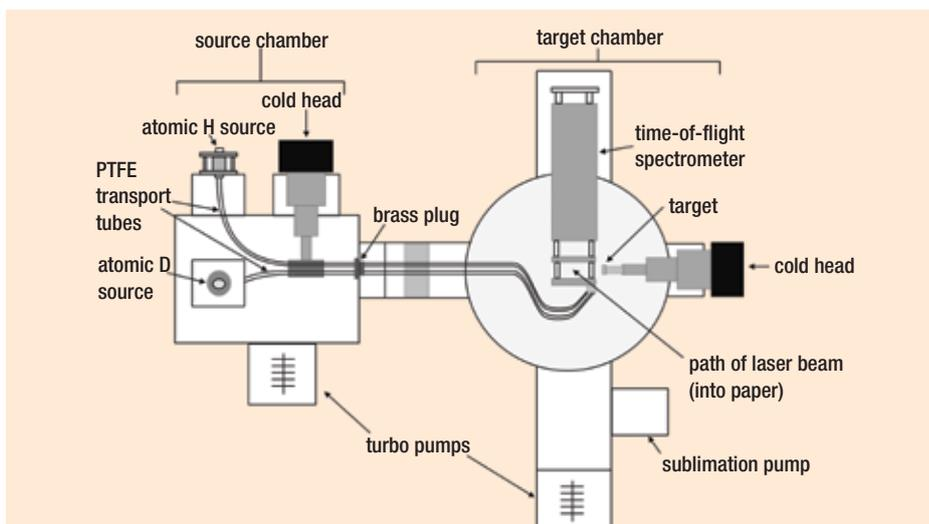
4: A schematic diagram of the UCL experiment to study the formation of  $\text{H}_2$  (HD) molecular hydrogen on cold interstellar surfaces using laser spectroscopy. H and D atoms from microwave discharges hit a cooled graphite surface. (Reused with permission from Susan C Creighan, James S A Perry and Stephen D Price 2006 *J. Chem. Phys.* 124 114701. Copyright 2006, American Institute of Physics)
